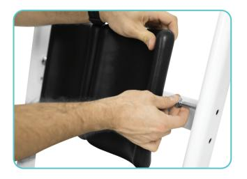
Place All four Small Bolts in the holes provided making sure they all sit flush and the square part of the bolt fits the square shape of the hole and the bolt end protrudes to the outside of the device.
