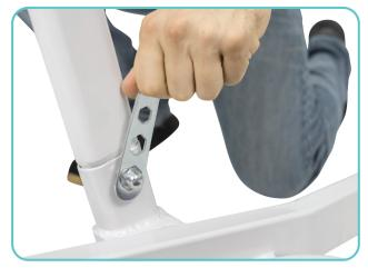
6. Use Small Bolt (F) to secure down both Base Posts (B) to the Base (A). Place the bolt in through both pieces from the outside so the bolt head sits flush, fits into the square shape and protrudes through to the inside of the device. On the inside of the device where the bolt is now sticking through, add first the Flat Washer (G) then the Locking Washer (H) and finally the Bolt Nut (I) and secure it on using the Hex Wrench (L).
