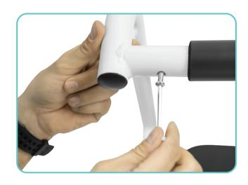
5. Use Small Bolt (F) to secure on both Right and Left Seat Arms (C,D) to the Base Posts (B). Place the bolt in through both pieces from the inside so the bolt head sits flush, fits into the square shape and protrudes through to the outside of the device. On the outside of the device where the bolt is now sticking through, add first the Flat Washer (G) then the Locking Washer (H) and finally the Bolt Nut (I) and secure it on using the Hex Wrench (L).
